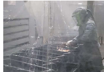
Grinding of newly cast parts
