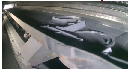
Casting exiting sand shakeout system
