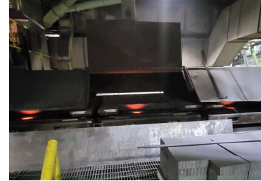
Casting cools in the mold for 2-4 hours
