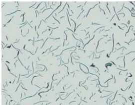
Cast gray iron microstructure
