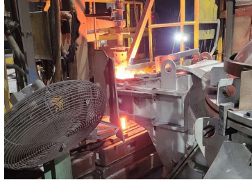
Molten iron is poured into the mold
