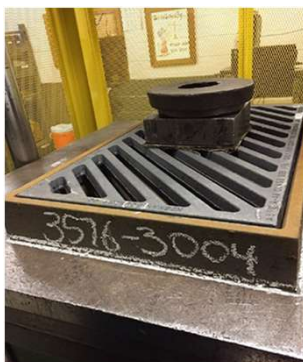
Grate and Frame Pre-Test Setup
