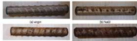
Figure 4-46: KM28 specimen (a) prior to testing and exposed to 50 cycles of (b) NaCl, (c) MgCl 2 , and (d) CaCl 2
