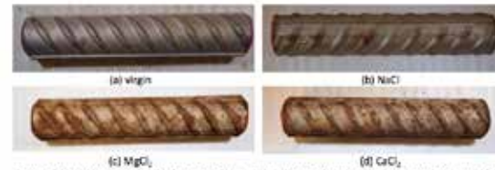
Figure 4-35: 304L specimen (a) prior to testing and exposed to 50 cycles of (b) NaCl, (c) MgCl 2 , and (d) CaCl 2
