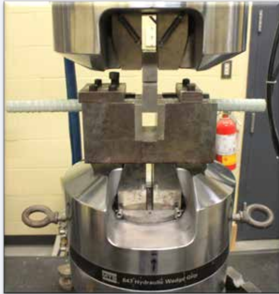
Shear Test Setup TRANSVERSE SHEAR STRENGTH BEYOND 220MPa IS MAINTAINED.
